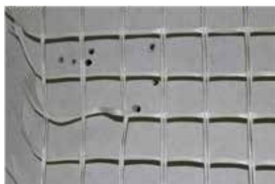
The fiber glass mesh does not deform permanently, but regains his form.
