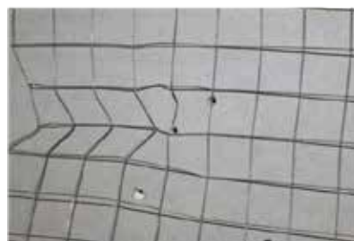
The galvanized net deforms permanently.
