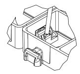
The interlocking system is strongin order to guarantee a perfect connection and stability on the entire surface. In case of unfastening of some grids, you need a tools that acts as a lever, such as a common flat head screwdriver. The process is very simple:
