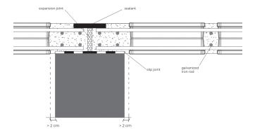
The designer must allow for at least **2-3 centimetres** between the load-bearing structure and the first row of glass blocks in the panel, in order to prevent the glass from coming into direct contact with the support.
