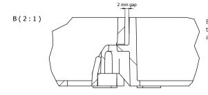
Each grid has a click interlocking system on aside, in order to connect the panels and to create a continuous surface, which become completely invisible once filled with aggregate, gravels or grass.
