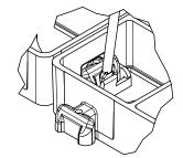
The interlocking system is strongin order to guarantee a perfect connection and stability on the entire surface. In case of unfastening of some grids, you need a tools that acts as a lever, such as a common flat head screwdriver. The process is very simple:
