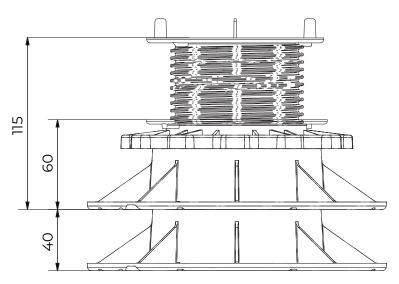
Each base has a special bottom shape that allows to be stack on another base.
