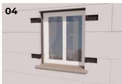
04 Complete the laying of the insulation.
