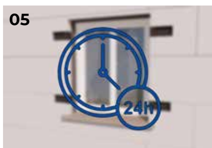
05 Wait 24 hours to allow the adhesive to fully adhere.
