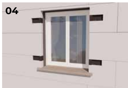
04 Complete the laying of the insulation.
