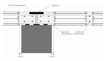
Horizontal Dakota glass elements must always be kept at a minimum distance of **3 cm from** the supports in order to avoid disregarded loads.
